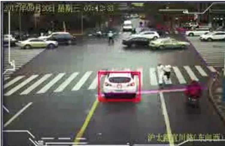
Fig. 24.2 A car breaching traffic law, automatically identified. Source The Author
