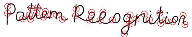
Fig. 5. Junction candidates in Fig. 2. The red points are the junction candidate center points. The red circles around the red points have no special meanings but improve visualization. (For interpretation of the references to color in this figure caption, the reader is referred to the web version of this paper.)
