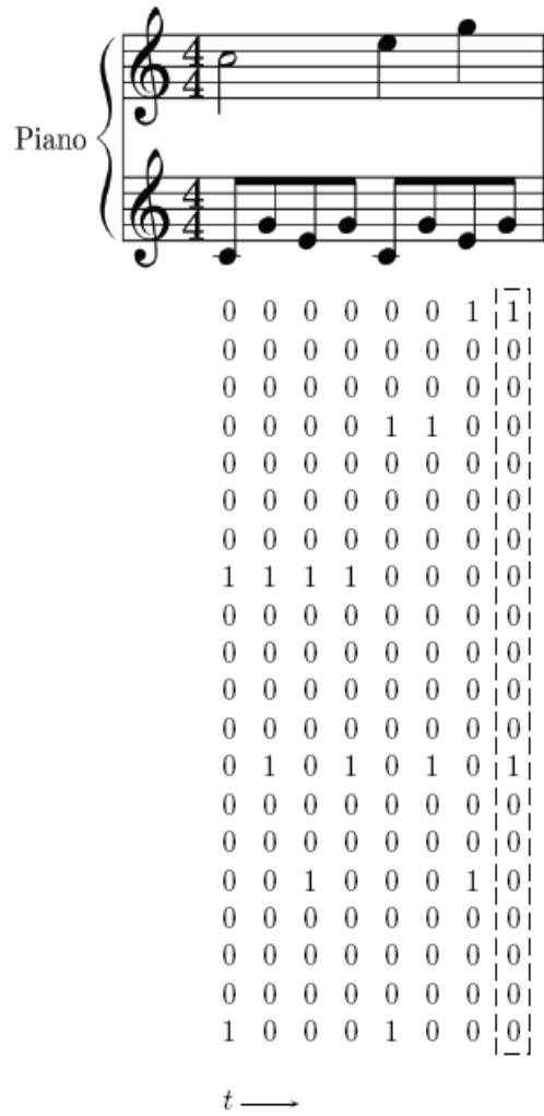
Figure 4.3: On the top the representation of a MIDI file in staff and under it, the representation for the RNN. The numbers in the dashed box represent one input pattern for the RNN in one timestep. The figure is taken from [16].
