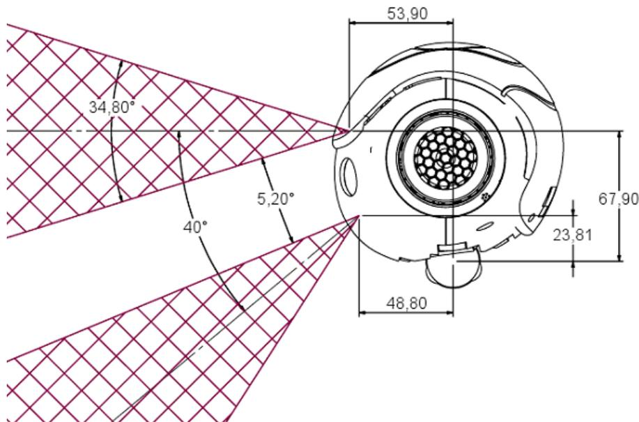
Figure 3.2: The placement of the cameras in NAO's head.
