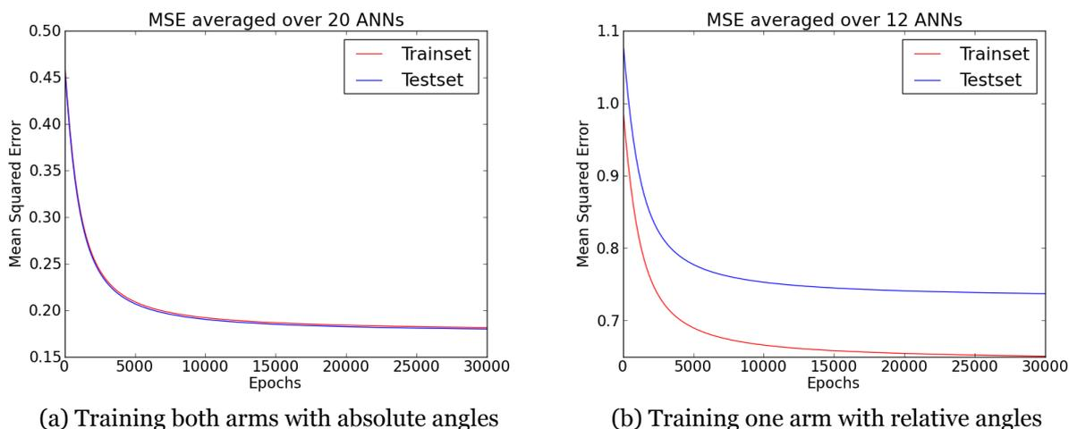
Figure 4.5: The MSE on the training set and the test set during training for 30000 epochs, for training on relative and absolute angles.
