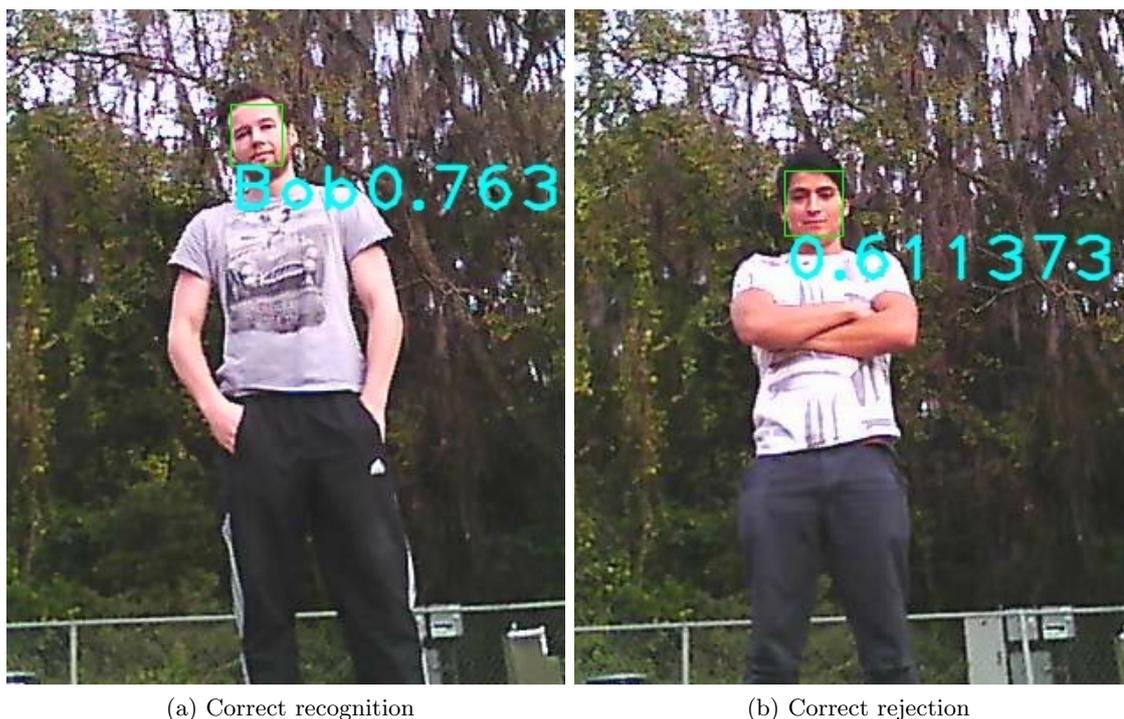
Figure 4.4: Examples from the facial recognition module on frames from a UGV
