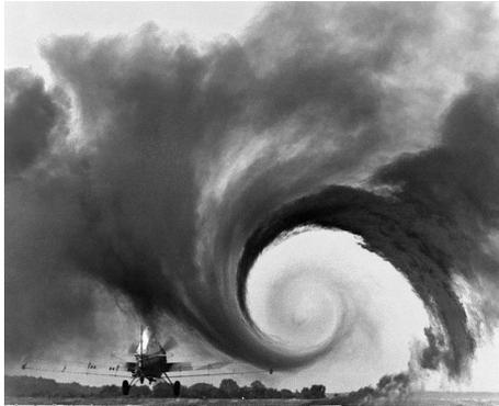
Figure 7: Wake vortex on an airplane, source: NASA Langley Research Center (NASA-LaRC)
