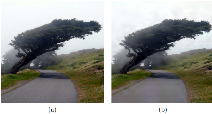
Figure 3.13: Sparse approximation of a natural image (a) Original image. (b) Approximation of the image obtained by keeping the largest 10% of the wavelet coefficients.
