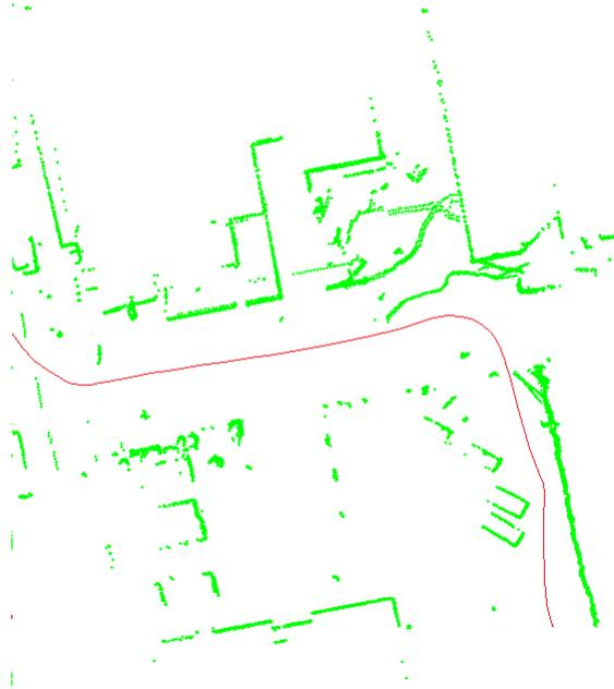
Figure 11: A map created using consecutive laser scans. The distance from left to right and up to down is about 50 meters and 400 scans were used. The length of the trajectory is about 90 meters.
