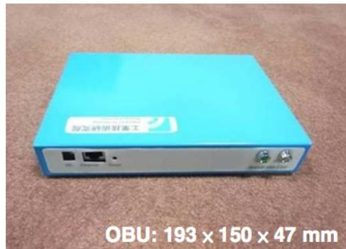
Figure 7: The DSRC module
