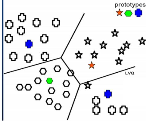
Figure 4: Example for LVQ with 3 Different Prototypes
