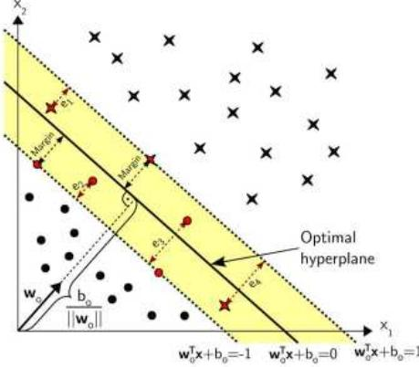
Figure 2: Linear Support Vector Machine. Function  $f(x)$  divides the feature space into two halves
