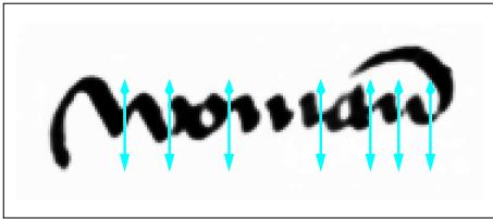
Figure 5. Handwriting segmentation at the minima in the upper contour that are proximal to the lower contour.
