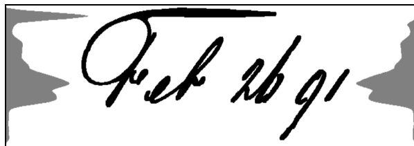
Figure 2: On the left is a standard projection profile, while on the right the ink run-length was used for normalization. Notice that the sharp top peak corresponding to the horizontal dash is eliminated.
