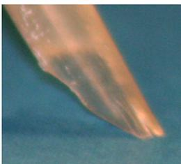
Fig. 4. A quill nib. The slit (incision) partly splits the nib into two tines; this enables width variation by changing pressure.
