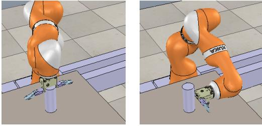
Fig. 3. *Left*: The end effector is sent to the center of the object which is permeable for demonstration purpose. *Right*: The predicted offset (5cm along y-axis, and 90 degrees around x- and around y-axis) is added.
