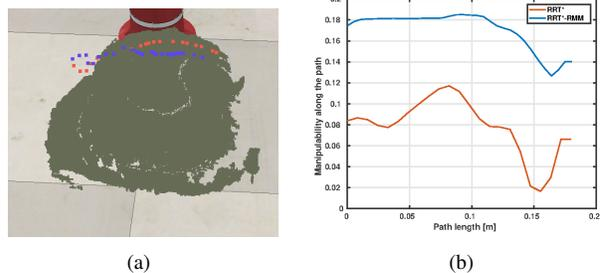
Fig. 1. The image shows the results of RRT\* (red) and RRT\*-RMM (blue) on a helmet. Fig.1(b) depicts the manipulability of the two paths. A little discrepancy between paths and pointcloud is due to visualisation purposes.
