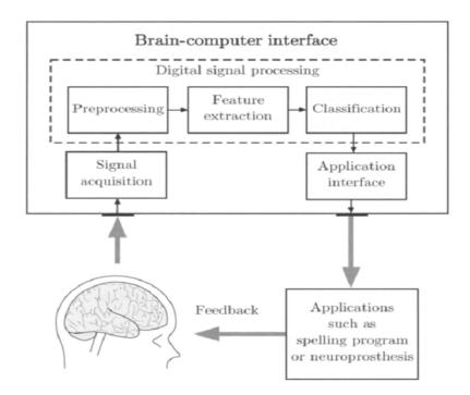
Figure 4-10: Block diagram of a typical BCI system [2].
