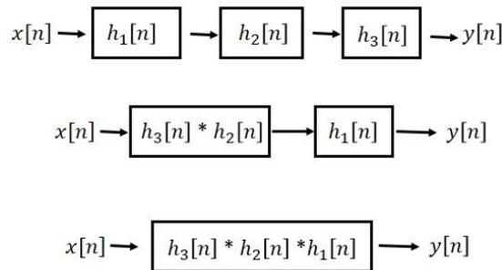
Figure 3-5: Three LTI systems with identical impulse response.
