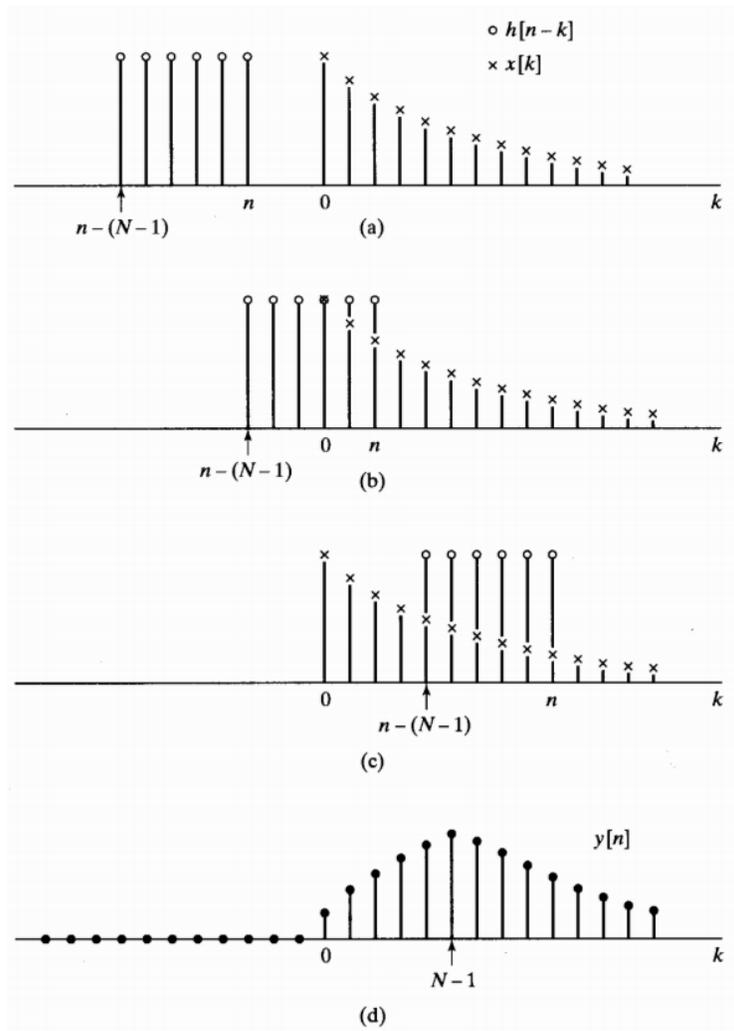
Figure 3-4: Sequences involved in computing the discrete convolution in example 3-2 [1].
