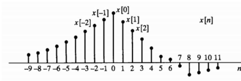
Figure 3-1: Graphical representation of a discrete- time signal [1].
