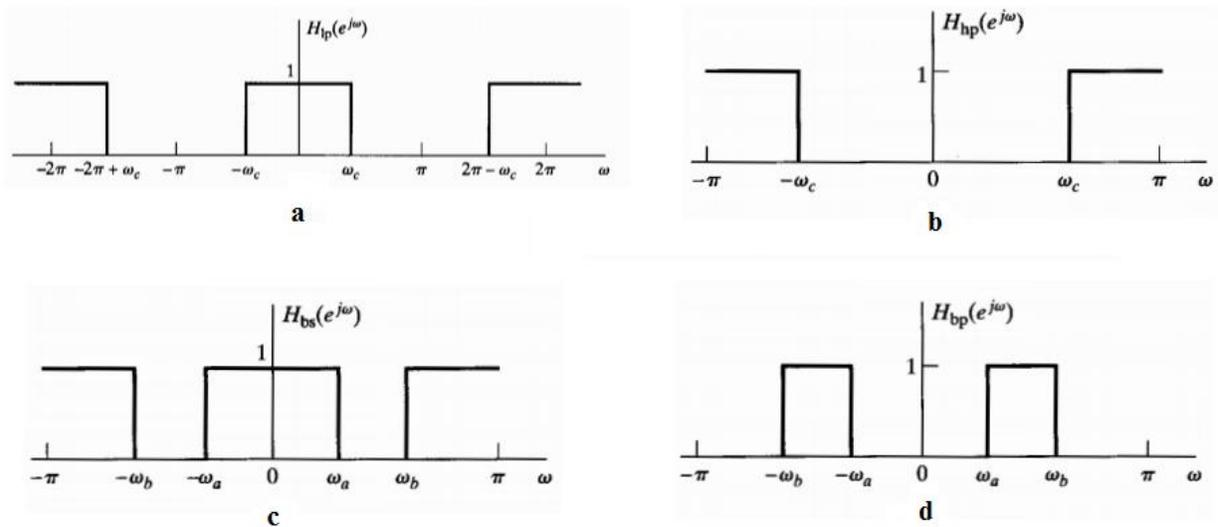
Figure 3-8: frequency response of ideal selective filters. a) low-pass, b) high-pass, c) band-stop and d) band-pass filters [1].
