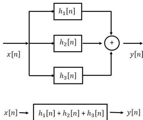
Figure 3-6: Parallel combination of LTI systems and the equivalent system.
