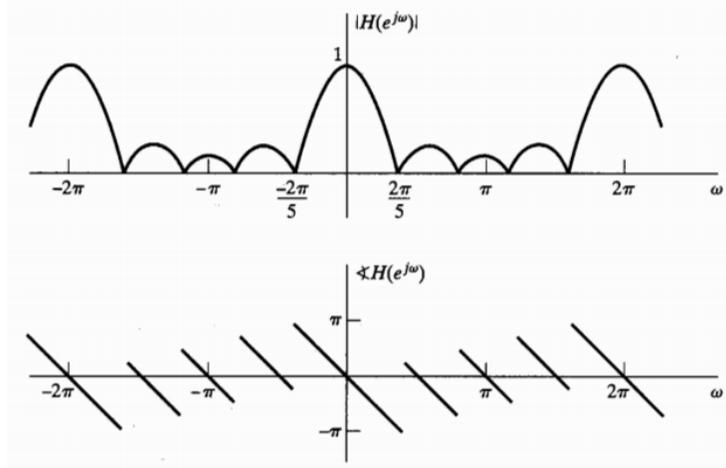
Figure 3-7: magnitude and phase of the frequency response of the moving average system with  $M_1 = 0, M_2 = 4$  [1].
