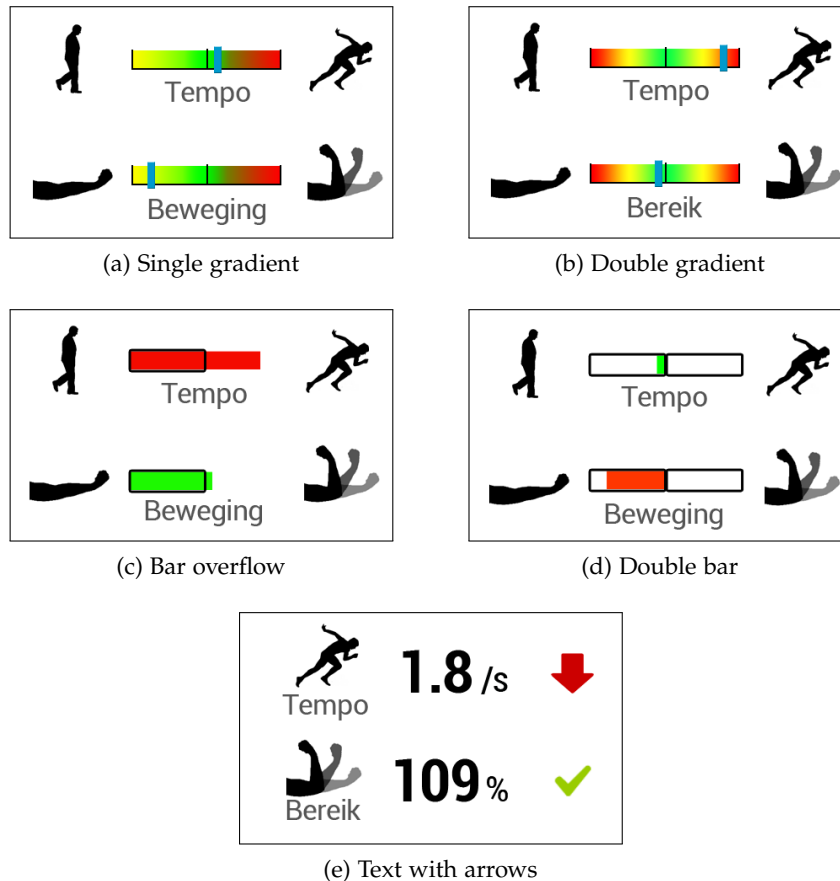
Figure 4.1: Five different display designs used in the display usability study. a) uses a yellow-green-red gradient to indicate a scale from too low to too high, where green is centered in the display and indicates the optimum. A blue rectangle indicates the user's performance. b) uses a double gradient to indicate that both extremes are undesired. c) uses the overflow metaphor, where a black outline indicates the optimum level and a bar indicating the user's performance can over- or underflow this bar. d) uses two bars of which one fills from the center outwards. e) shows the values corresponding to the properties. Values larger than 100% are too high and under 100% too low. The word 'bereik' and 'beweging' are Dutch for range and movement, respectively.
