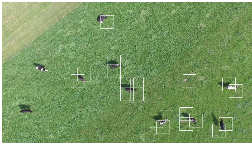
Figure 5.3: (Poor) detection in a video frame. The image shows mistakes where the detector does not recognize a cow (left) or recognizes a patch of grass as a cow (right). Also it is clear that due to the sliding window approach patches of ground around the cows are detected.
