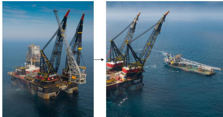
FIGURE 2.8: Photo of a real execution. (Left) suspended module on crane. (Right) Module on barge for transport. [Photo: Bo B. Randulff og Jan Arne Wold/ Equinor.]
