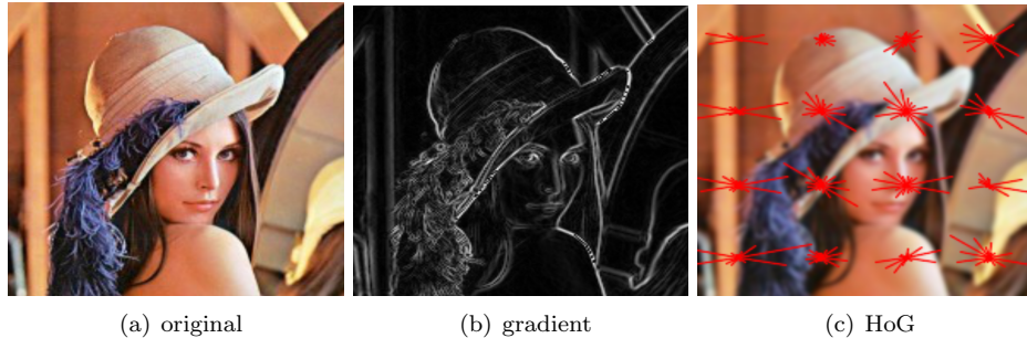
Figure 3.1: A visualisation of an image (a), its gradient and the HoG description computed from that gradient. The image gradient visualisation (b) is white at high magnitude areas emphasizing edges and noisy areas. Along with these magnitudes, an orientation for each pixel is calculated, not visualized in this image but it is visualized indirectly in the HoG descriptor visualisation (c). To calculate the HoG description, the image gradient is divided regularly into a number of rectangular regions. In this example the image was divided into 4 \times 4 = 16 areas for the sake of visibility, for the actual description however it is divided into 8 \times 8 = 64 segments. In (c) these histograms are visualized by a set of vectors for each histogram. Every region has 16 vectors, each representing a bin of the histogram, the length of that bin representing the magnitude in that direction within the area.
