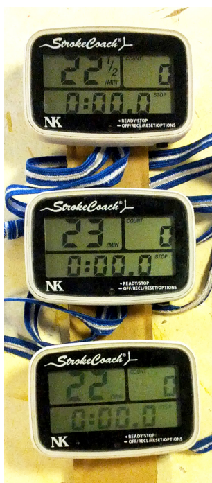
Figure 12: Three StrokeCoaches with Surge Rate Technology displaying different SPM while moved together
