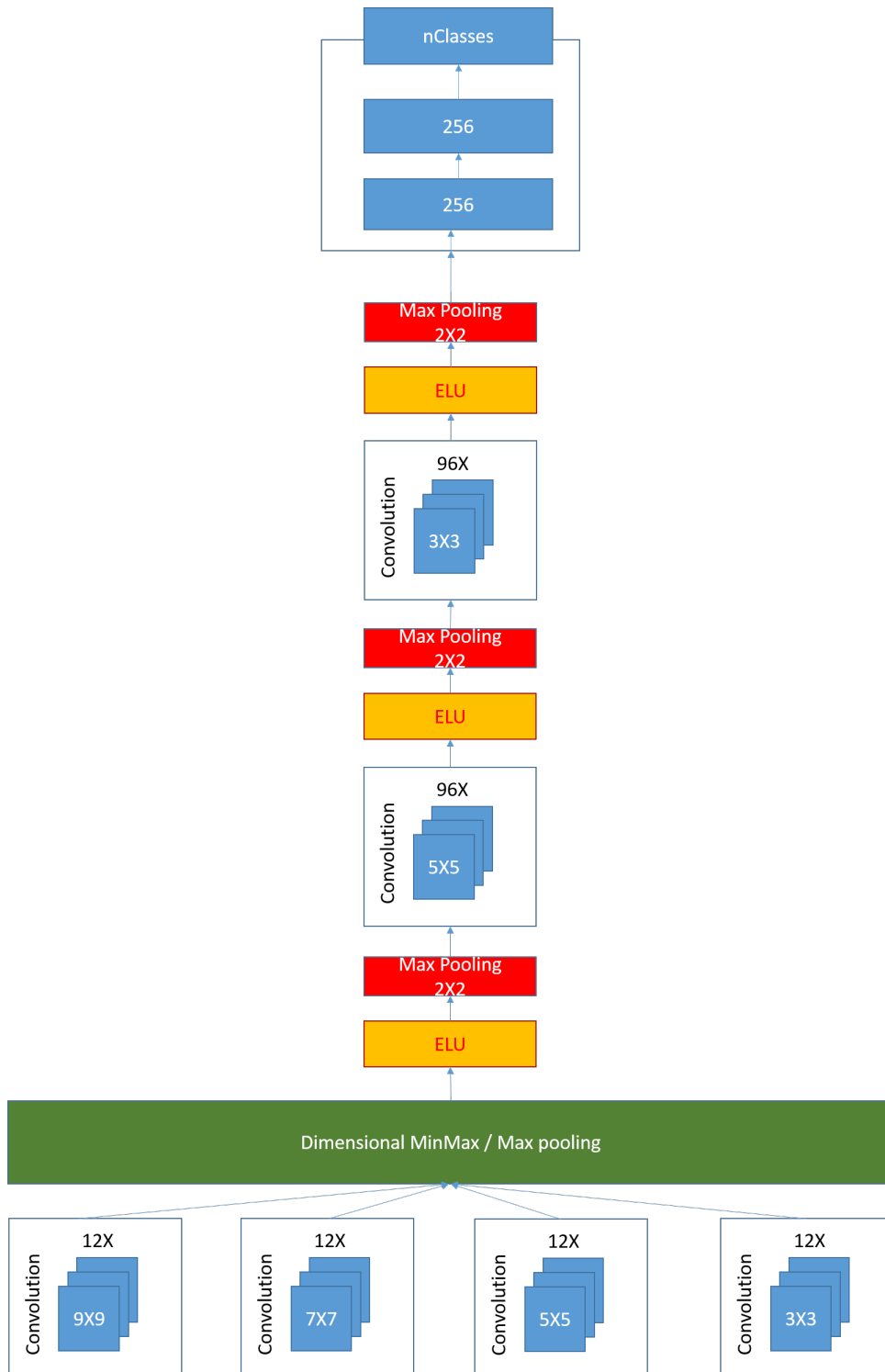
Figure 5.6: Structure of the Max/MinMax implementation used for the Cifar-10 dataset.
