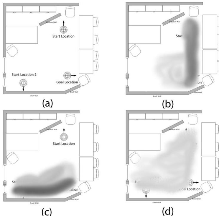
Figure 15 Scenario 1. (a) Start and Goal Locations. The arrows show the used direction to start or finish. (b) Trail of the robot using neural gas and value iteration from first start location. (c) Trail of the robot using neural gas and value iteration from second start location. (d) Trail of the robot using random search
