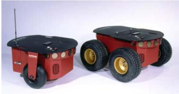
Figure 11 (left) Pioneer 2 Platform (right) Pioneer 2 AT Platform
