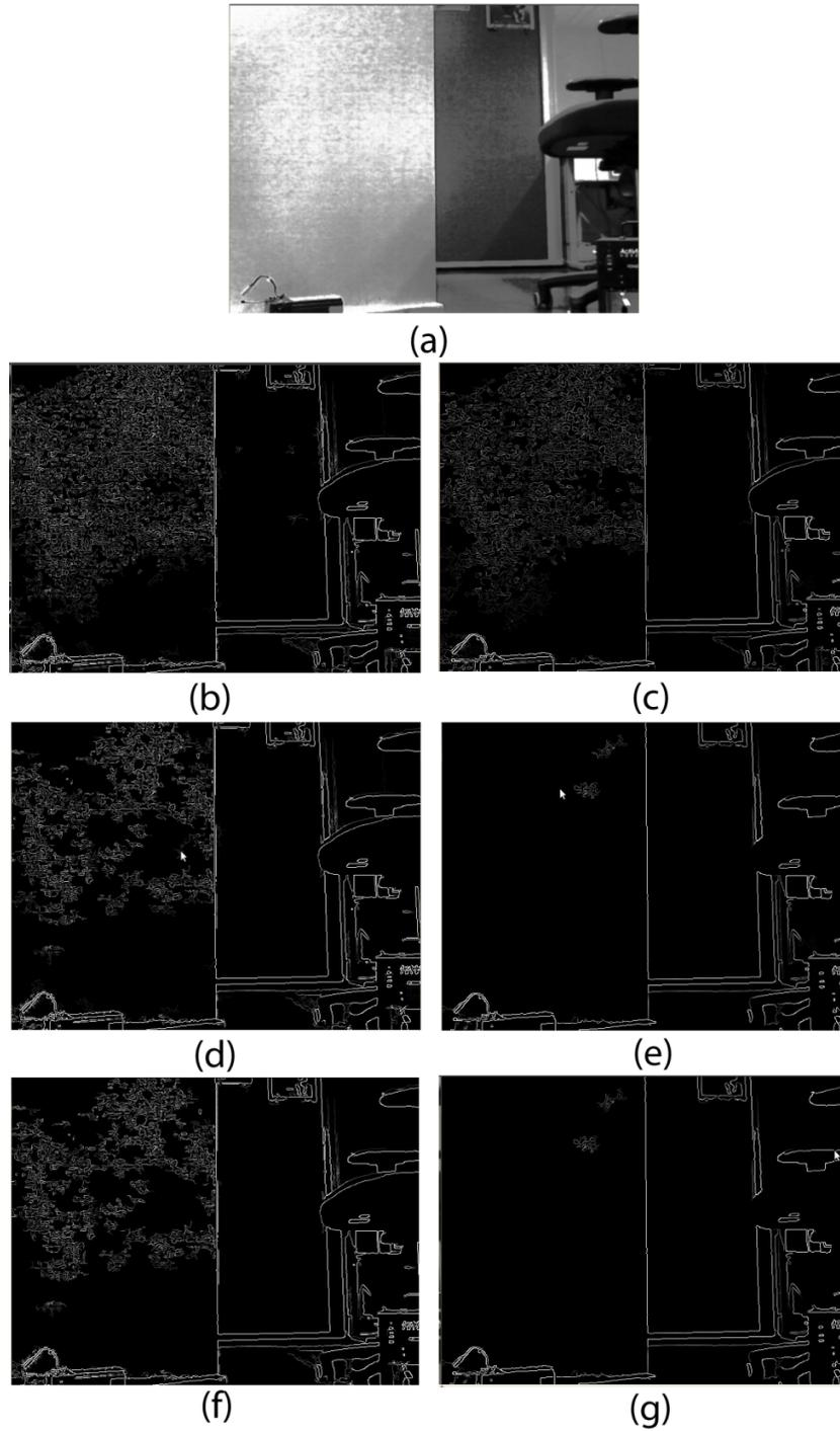
Figure 14 Canny edge detector results with different parameters (a) Original Image. (b) Threshold 1 is 1, threshold 2 is 128 and no smoothing. (c) Threshold 1 is 1, threshold 2 is 128 and with smoothing. (d) Threshold 1 is 1, threshold 2 is 255 and no smoothing. (e) Threshold 1 is 1, threshold 2 is 255 and with smoothing. (f) Threshold 1 is 30, threshold 2 is 250 and no smoothing. (g) Threshold 1 is 30, threshold 2 is 250 and with smoothing.
