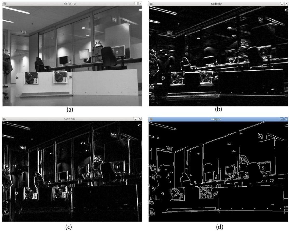
**Figure 7 (a) The original Image (b) The gradient image in direction y (c) The gradient image in direction x (d) The final Canny edge image**
