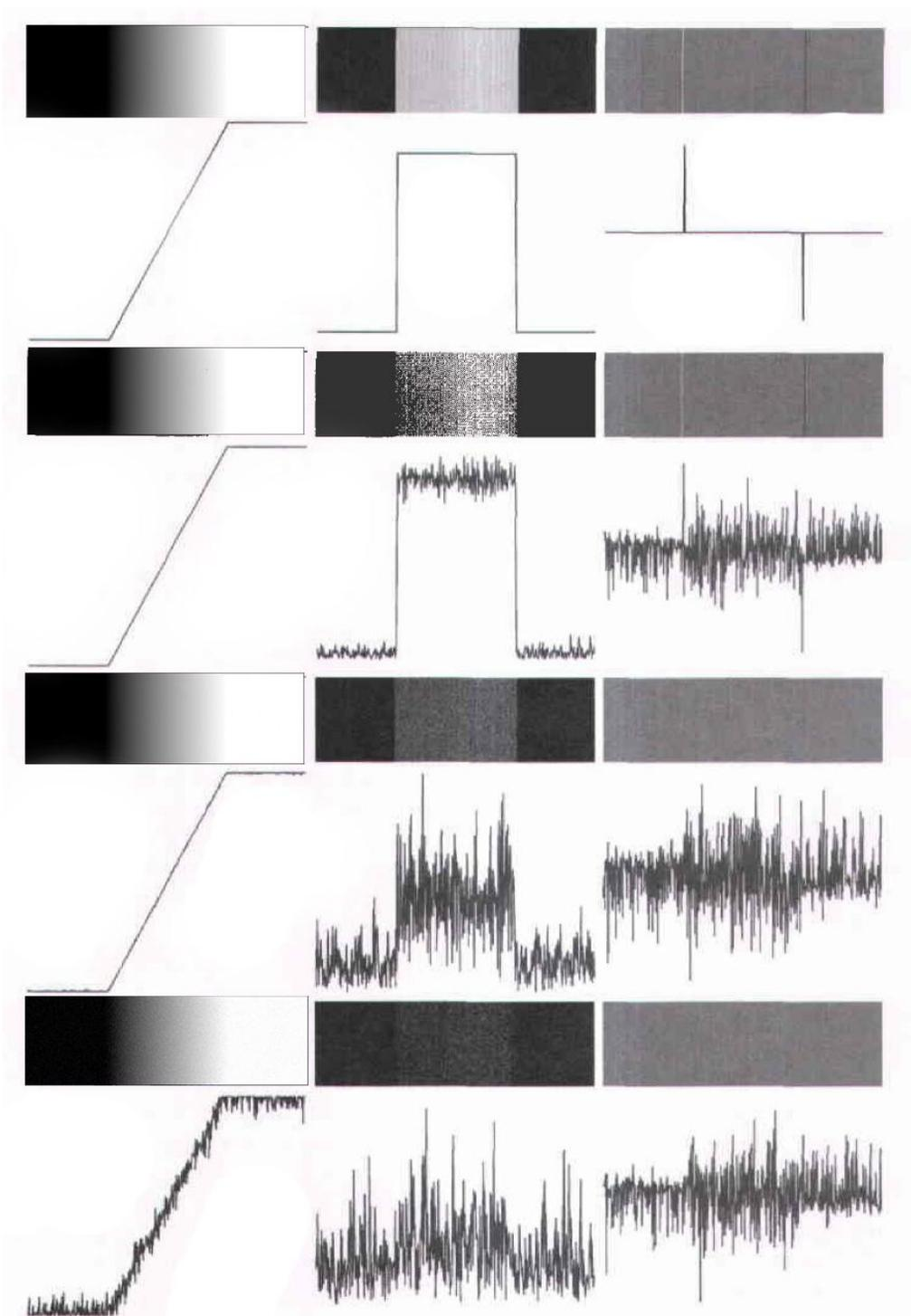
Figure 6 Four different ramp edges transiting from a black region to white region. The 2<sup>nd</sup> to 4<sup>th</sup> ramp edges are corrupted with additive Gaussian noise with zero mean and standard deviations of 0.1, 1.0, and 10.0 intensity levels. The second column is the first derivative. The third column is the second derivative. From the Image courtesy of Rafael C. Gonzalez.
