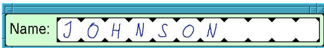
Figure 2: Typical dialog box, prompting for isolated handwritten characters. Although the quality of elicited character shapes is improved, this mode of data entry may be slow and tedious, especially if the recognizer (still) does not classify the characters correctly. For each dialog box, advance knowledge on allowable input may be used by the handwriting recognizer to improve the classification accuracy.
