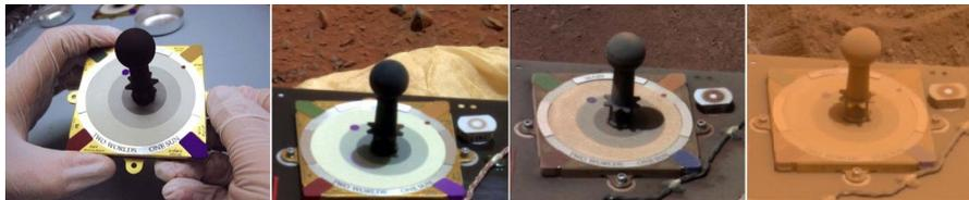
**Figure 9.1** Unexpected dust accumulation on the color calibrator of a Mars rover. Without actuators for autonomous self maintenance, only the wind can help out [KinchMarsDust, 2007].
