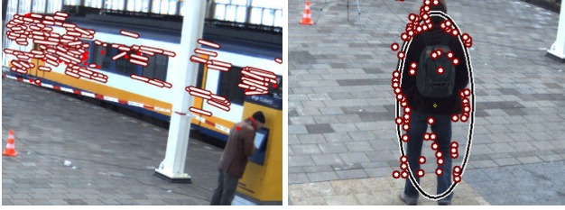
Figure 2: (Left) Optical-flow features for detecting trains in motion. (Right) Representing people: ellipses (for tracking) and points (for articulation features).
