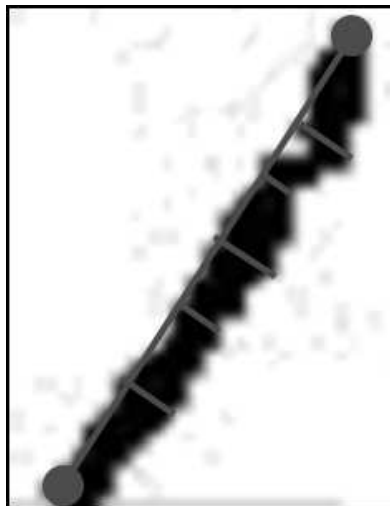
Figure 10: The object responsible for misjudging the bottom edge, enlarged and with marked orientation and perpendicular width measurement.
