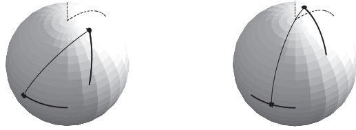
Figure 5.9: Maximum distance between two arcs. In the right picture, an endpoint of one arc is in the antilune of the other arc.
