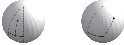
Figure 5.4: Minimum distance between a sphere point and an arc. In the left picture, the point is in the lune of the arc; in the right picture, it is not.
