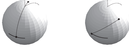
Figure 5.6: Maximum distance between a sphere point and an arc. In the left picture, the point is in the antilune of the arc; in the right picture, it is not.
