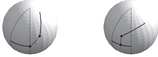
Figure 5.8: Minimum distance between two arcs. In the right picture, an endpoint of one arc is in the lune of the other arc.
