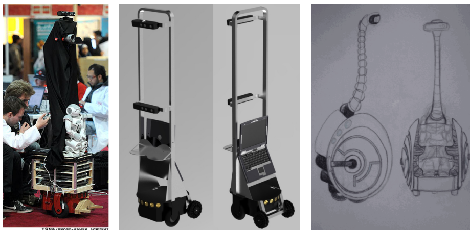
Fig. 1. ( Left ) Our previous prototype at the Iran Open 2011 competitions, a combination of a Nao and a Pioneer robot. ( Middle ) Our current prototype design for the Robocup@Home 2012 competitions with additional omni wheels for higher load capacity. ( Right ) Concept art of the final design.
