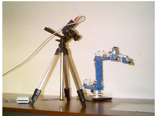
Figure 1: The experimental set-up, consisting of a stereo head and a robot arm.
